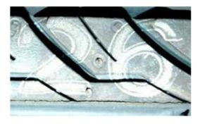
When a tyre is being assembled, all the components are put together (carcass, beads, belts etc) inside a tyre mould and the stripes help the technician to align the tread stock properly.
