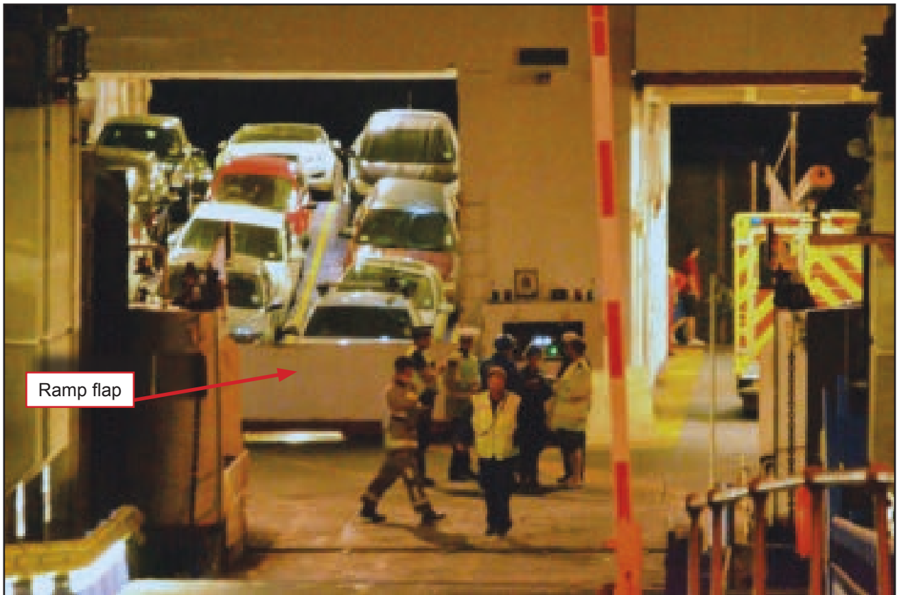
Figure 6: Outboard side of mezzanine deck lowered to main deck level
