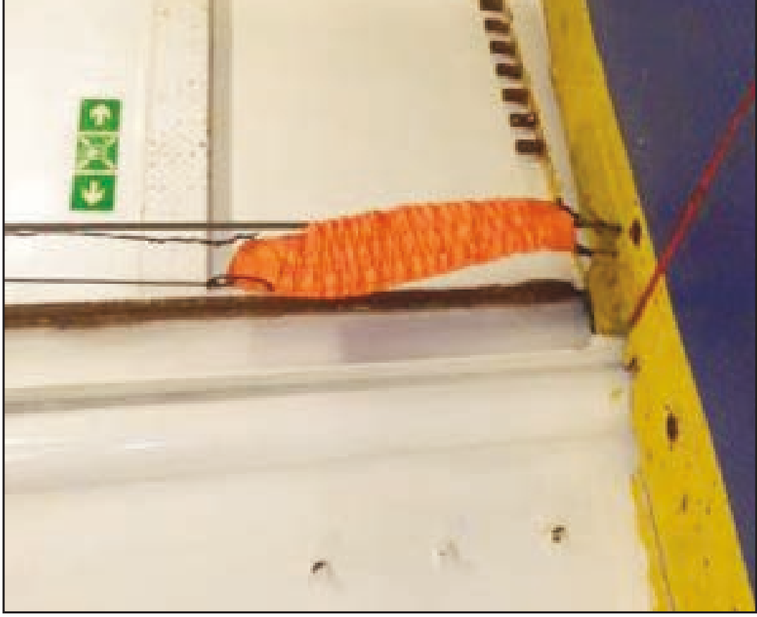
Elasticated lifting rope grease guard on board St Claire
