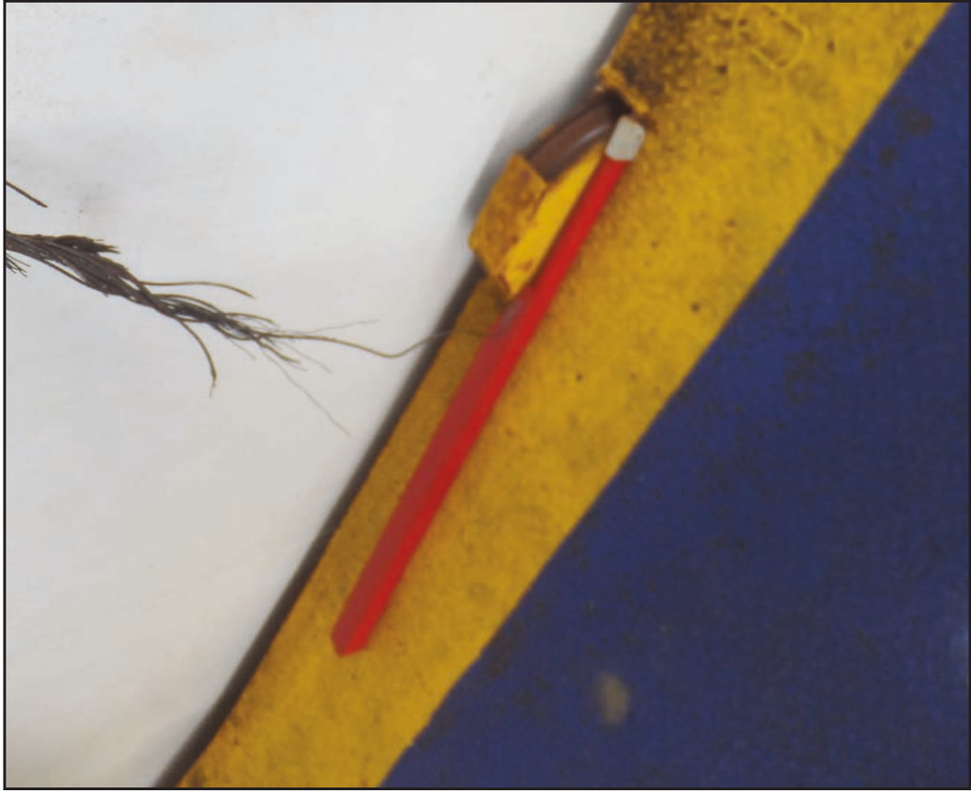
Hinged wooden lifting rope grease guard on board St Helen
