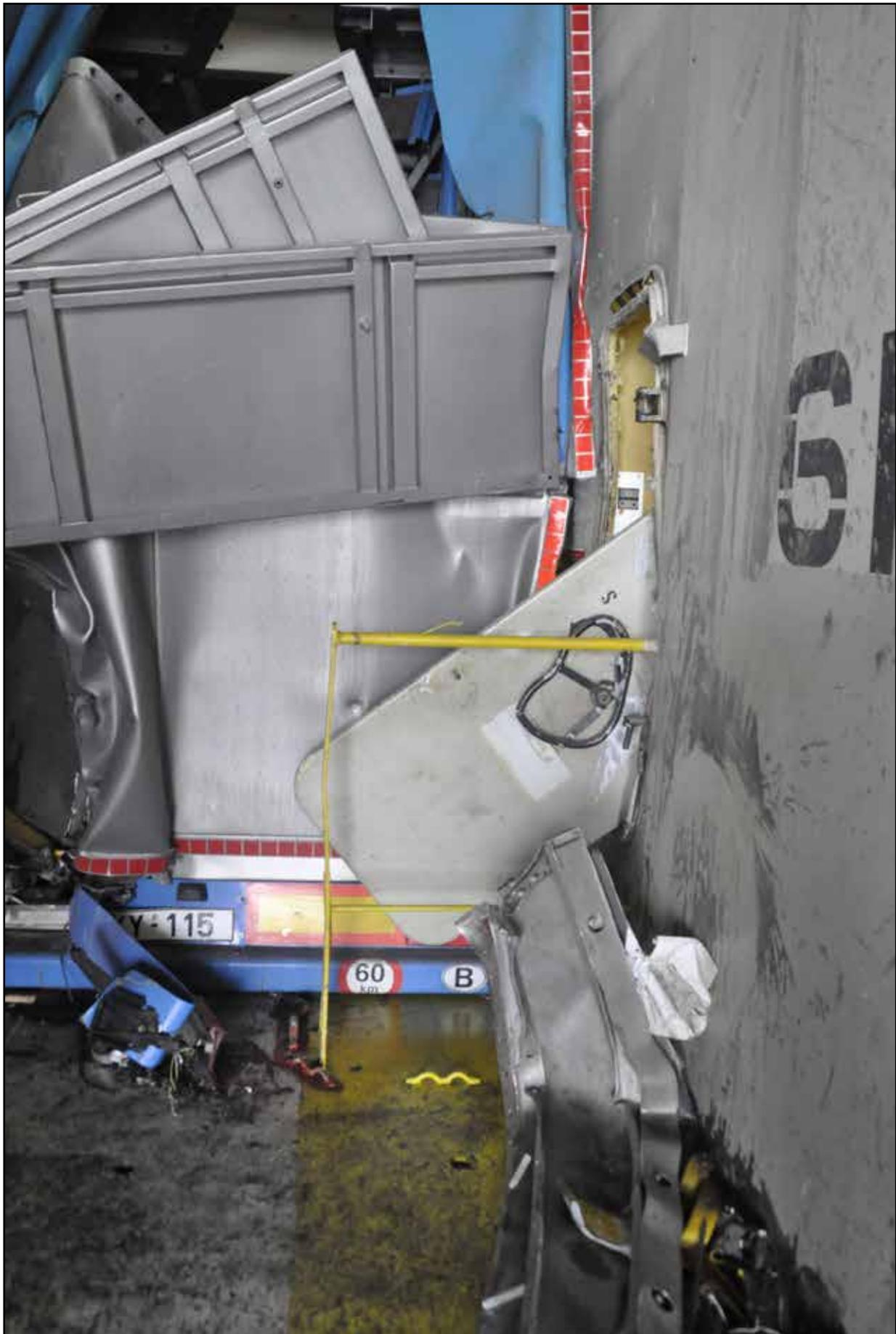
**Figure 11:** Damage to starboard side of deck 6 caused by moving cargo
