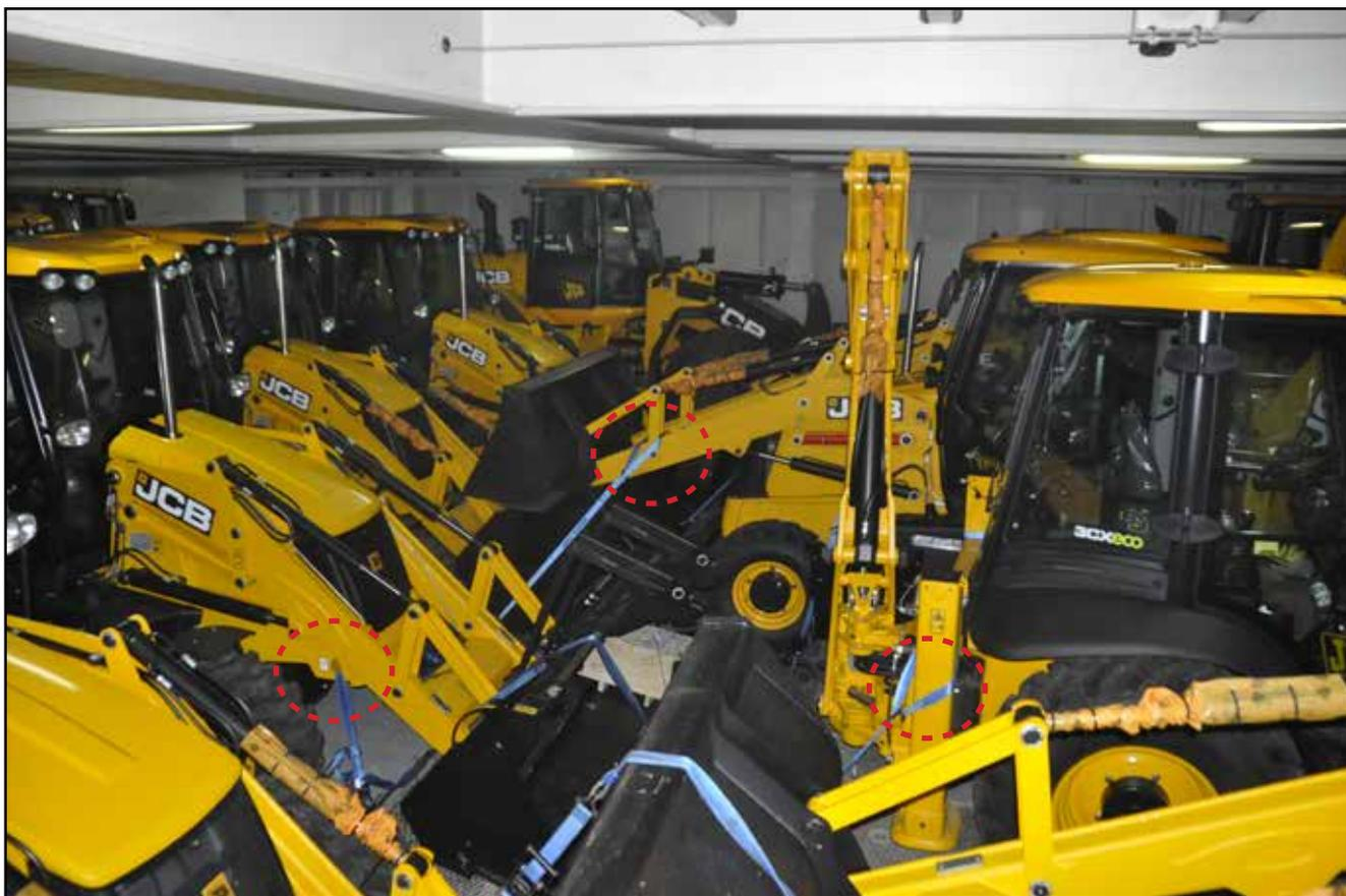
**Figure 27:** JCB cargo indicating various securing points
